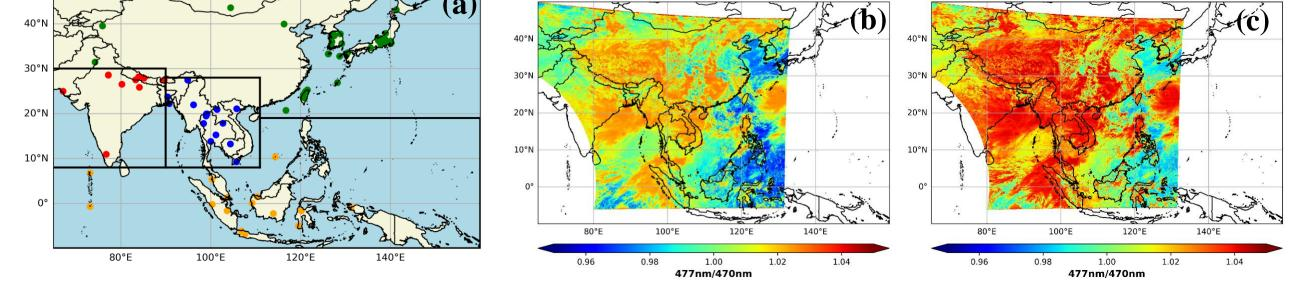
(a) Regional LUT, (b) Normalized radiance ratio of 477nm to 470nm using 2.2nm binning, (c) using 1.1nm binning
