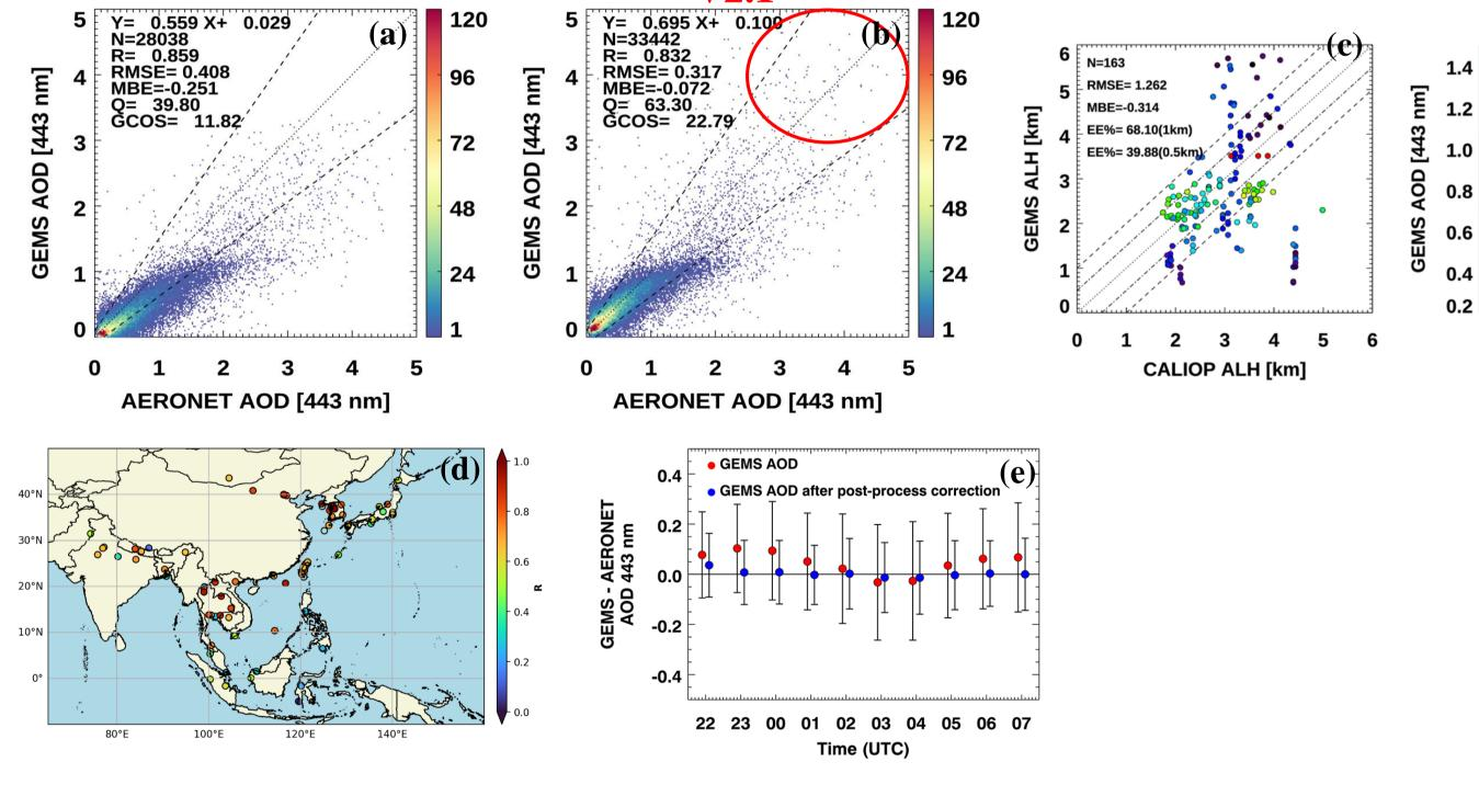
(a)~(b) Comparison of GEMS AOD and AERONET AOD from January 2023 to May 2024 (c) Comparison of GEMS ALH and CALIOP ALH from November 2021 to October 2022 (d) R-value of validation results for GEMS AOD v2.1 from January 2023 to December 2023 (e) Diurnal bias of GEMS AOD after post-process correction (Cho et al., 2023)
