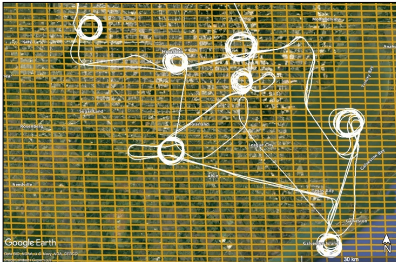
Figure 4-9 Example flight lines for collecting and deriving in situ column densities include aircraft spirals, low-altitude approaches over airports, or sets of vertically stacked flight lines.
