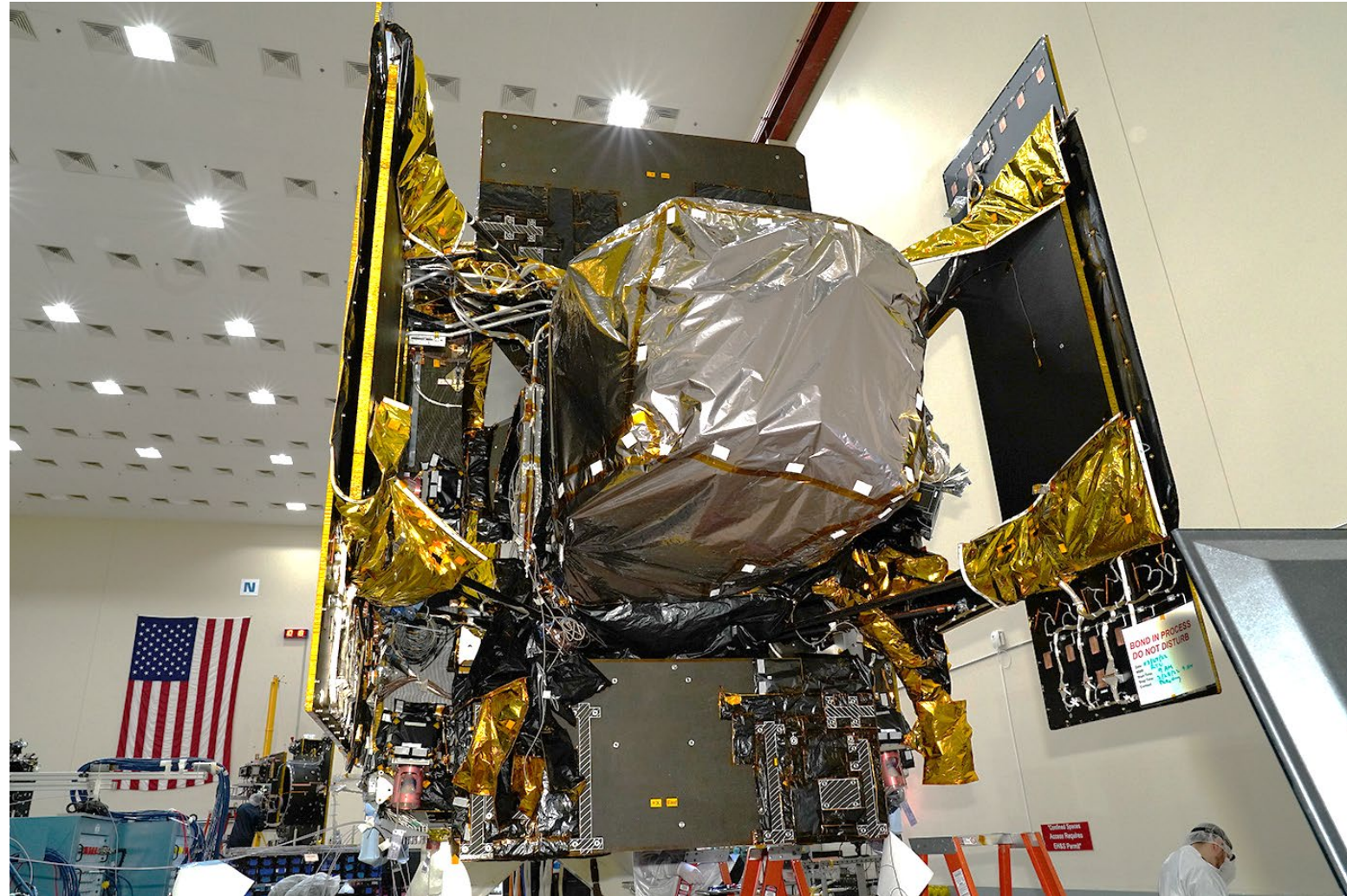
IS40e and TEMPO with purge bag viewed from Earth facing side
