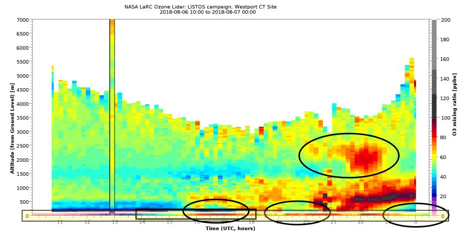
Ozone LIDAR data at Westport provides us with an encompassing snapshot of processes related to ozone production and ozone exceedances along the CT coast.
