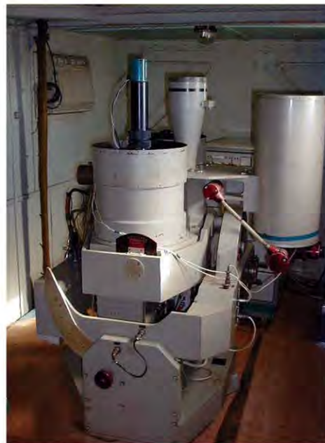
FIG. 1. Maket-1 lidar system installed at Camagüey in 1988.
